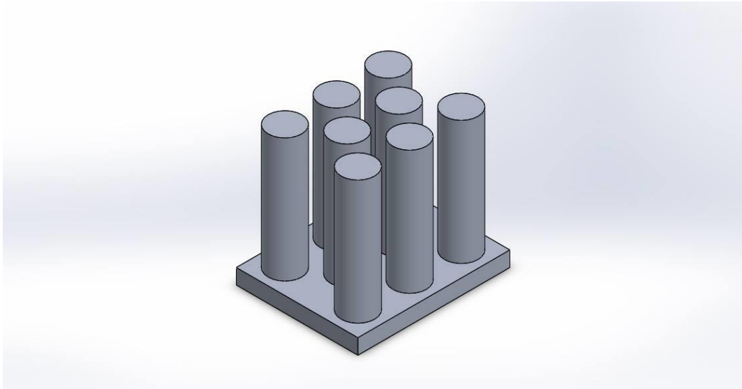
Figure 3.32: Solid works design of solid pin fin
