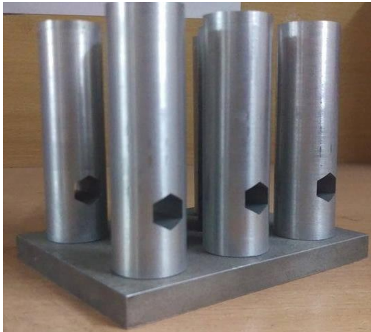
Figure 3.12: Pin fin with hexagonal perforation
