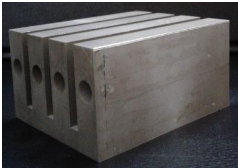
Figure 3.8: Plate fin with circular perforation
