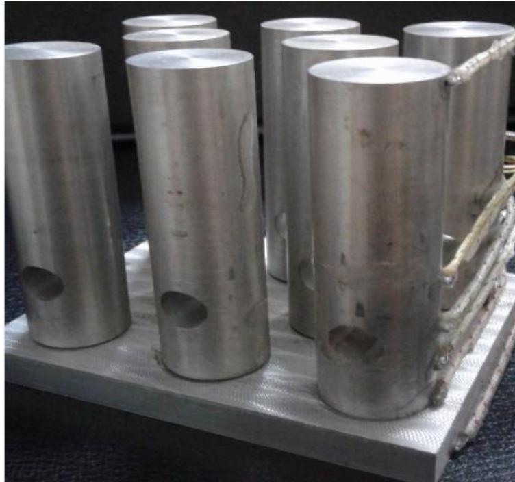
Figure 3.11: Pin fin with circular perforation
