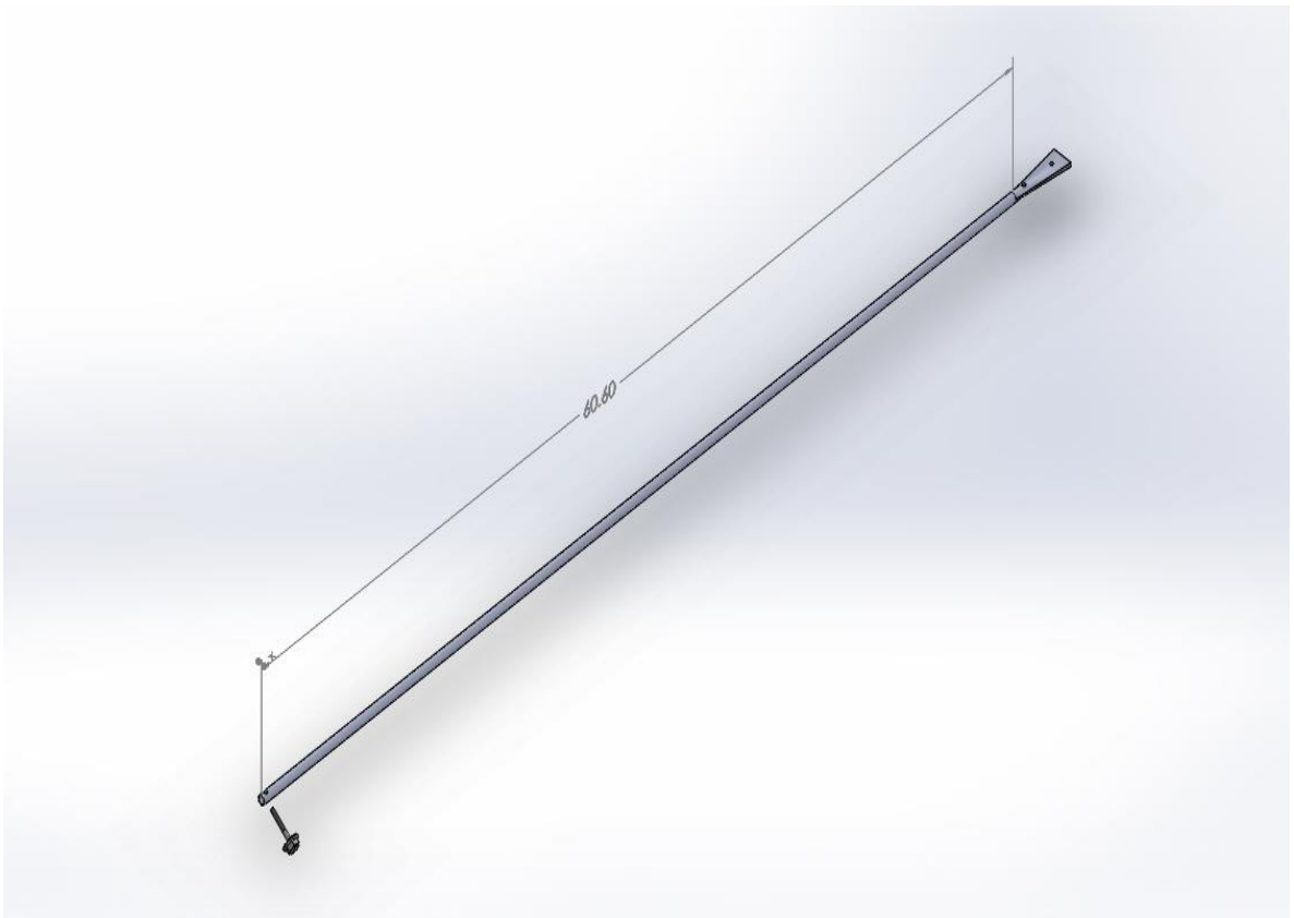
Figure 5.13: Single Rotor Arm with Dimension (dimensions in inch)
