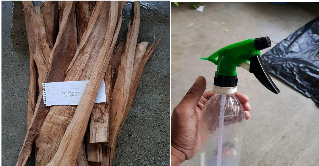
Figure 3.1: Spraying water on a section of biomass fuel to change moisture content
