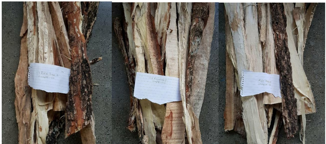
Figure 4.2: Raintree wood samples with varying moisture (wet, medium wet and dry from left to right)
