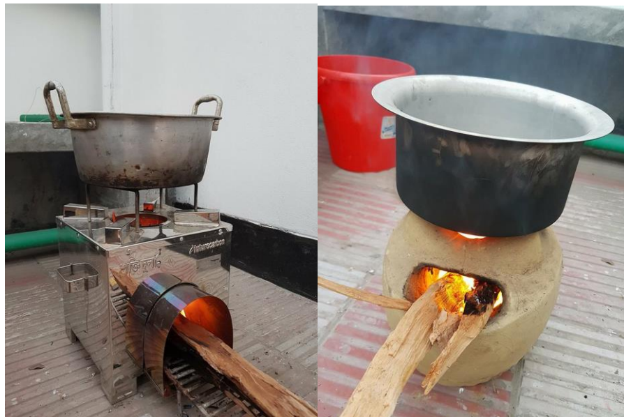
Figure 4.4: Experimental setup of cook stove. ICS (left), traditional (right)
