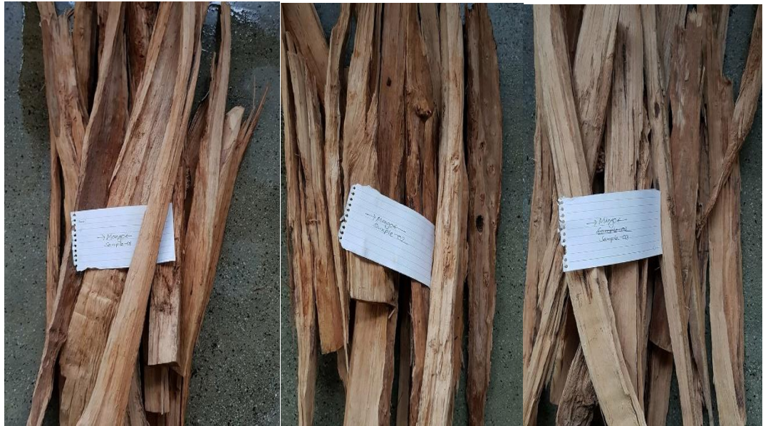
Figure 4.1: Mango wood samples with varying moisture (wet, medium wet and dry from left to right)
