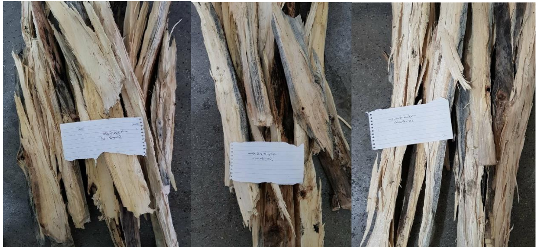
Figure 4.3: Jackfruit wood samples with varying moisture (wet, medium wet and dry from left to right)
