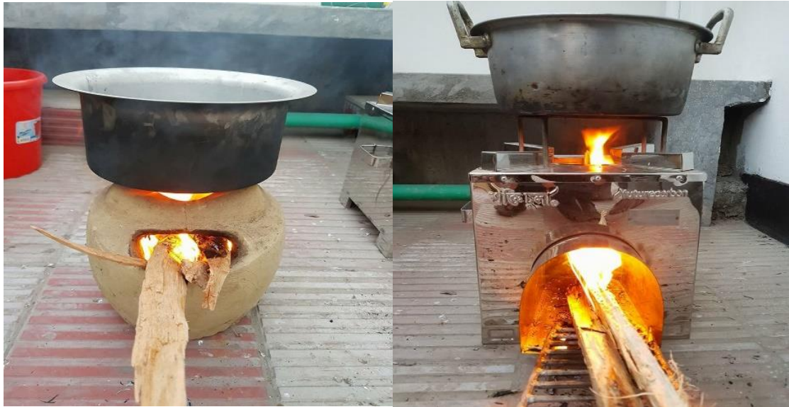
Figure 3.2: Boiling water in traditional stove and improved cook stove
