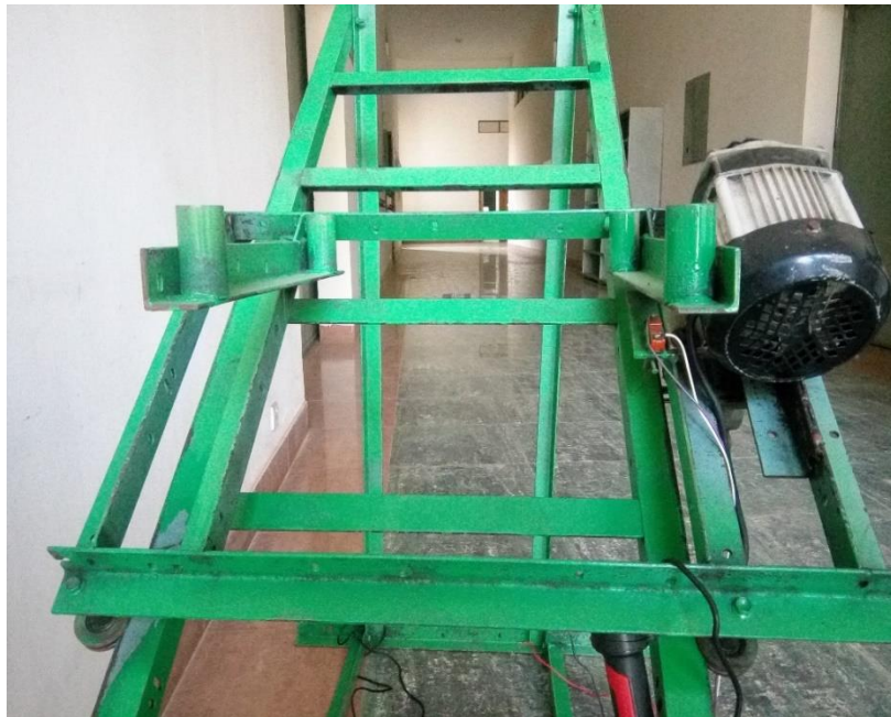
Fig 4. 4: Rail and carriage assembly
