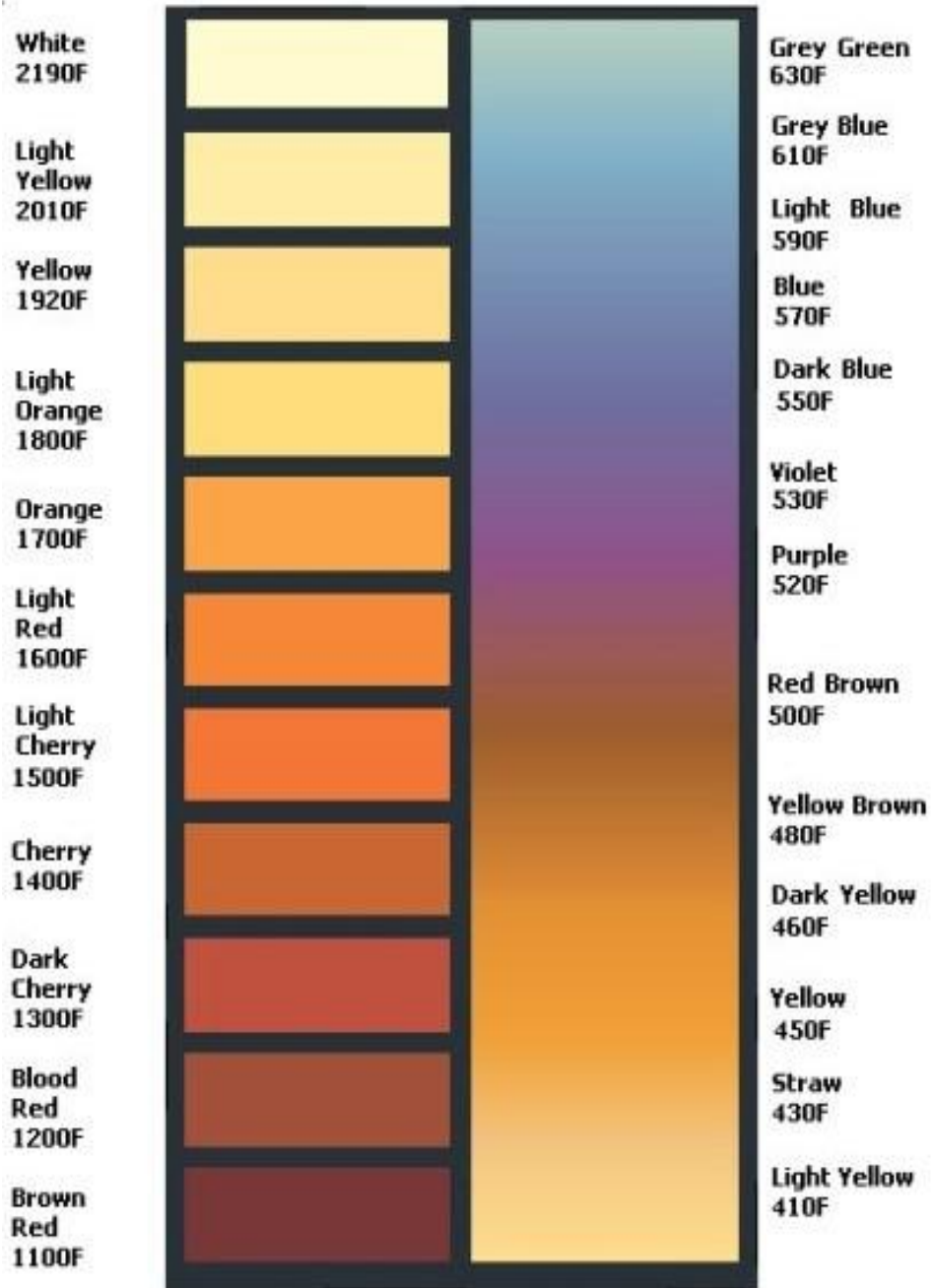
Fig 7.7: Heat treatment at different Temperature
