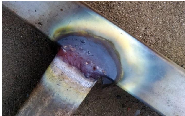
Figure 33: Arc welded joints
