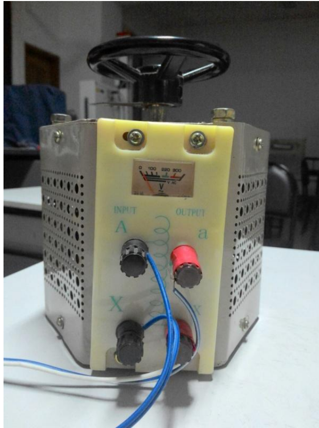
Figure 3.24: variable voltage regulator
