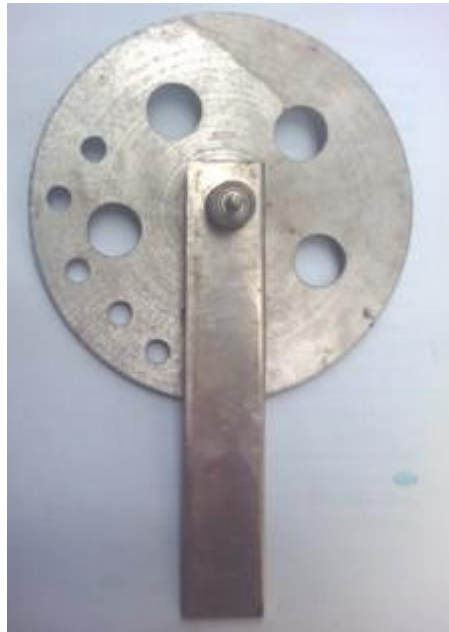
Figure 3-7: Fly wheel stand with a flywheel attachment
