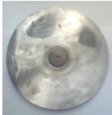
Figure 4-10: Flywheel after manufacturing
