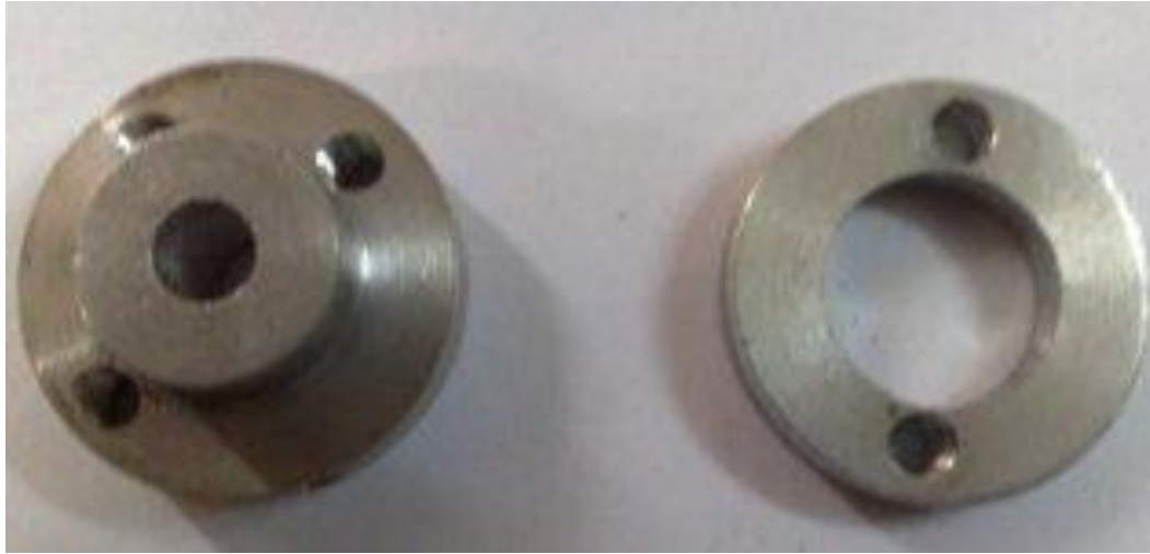
Figure 4-8: separate removable parts of flywheel
