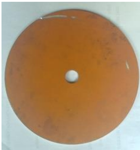
Figure 3-13: Flywheel before attachment
