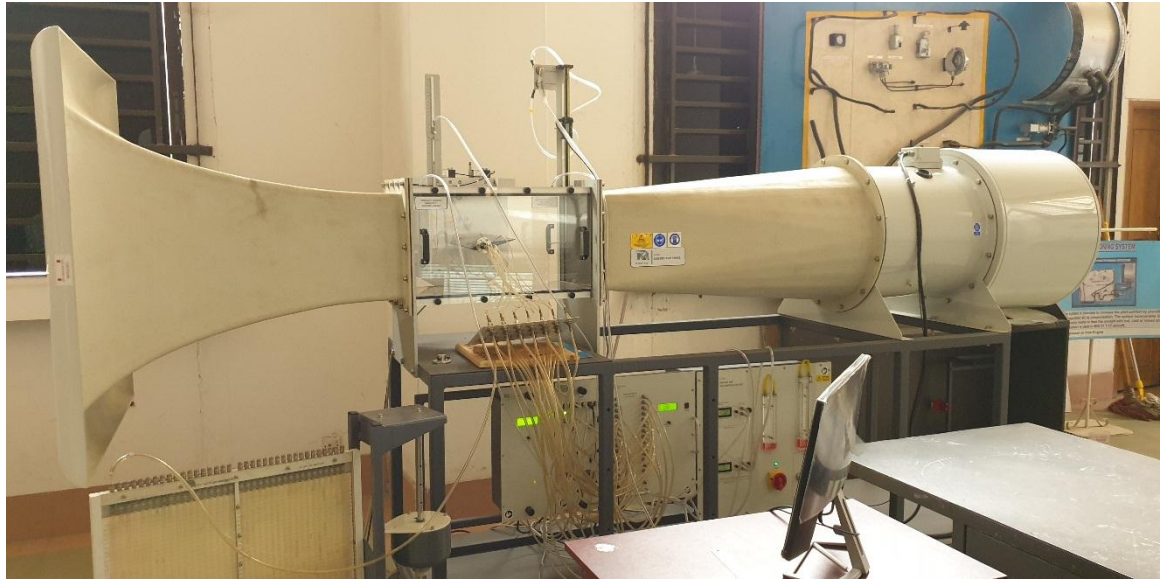
Fig. 6.2 Pictorial view of AF1300s subsonic wind tunnel
