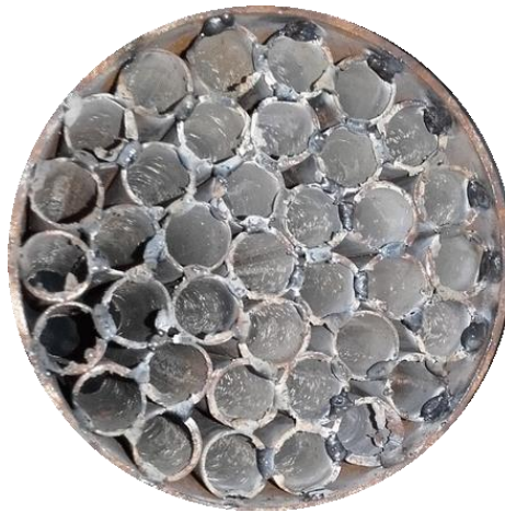
Figure 4.6: Honey Comb Structure (Inside Straightener)
