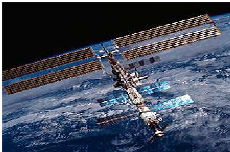
Fig: 2-21. PV on the International Space Station
