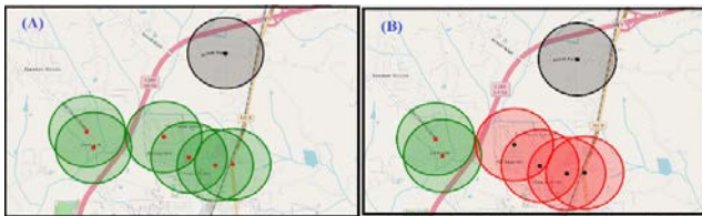
Figure 6. Clustering results from Sklearn’s DBSCAN function. (a) Shows results before converting to radians, and (b) shows the results after converting to radians
