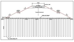
Figure 8: Cross section of embankment with Cement Mixing Piles.
