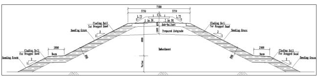
Figure 5: Typical cross section of embankment with height  $\ge$  4.0 m
