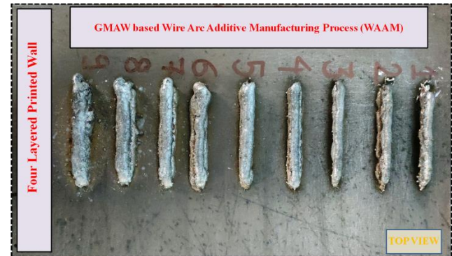
Figure 2: Fabricated WAAM specimens with different Heat Inputs
