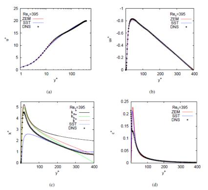
Figure 1: Mean profiles of turbulent channel flow at  $\text{Re}_{\tau} = 395$ : (a) velocity; (b) Reynolds shear stress; (c) k; and (d)  $\varepsilon$
