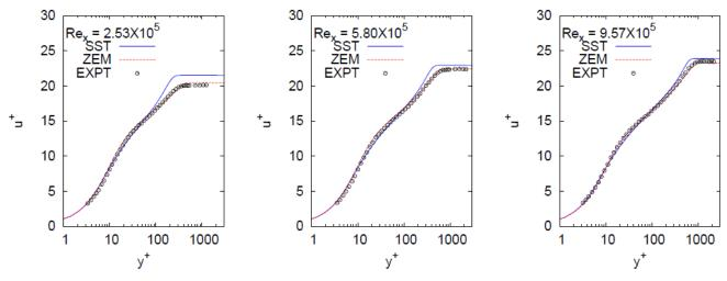
Figure 5: Mean velocity profiles for flat-plate at various downstream locations
