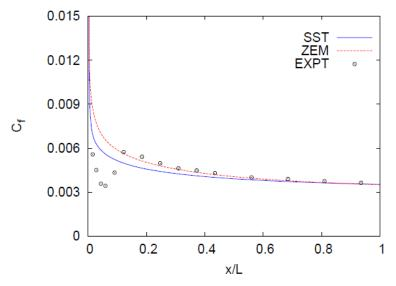
Figure 4: Skin-friction profiles for flat-plate BL case
