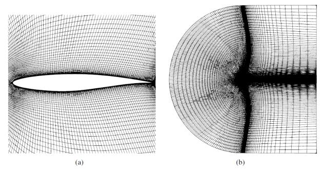
Figure 8: Computational grid for RAE2822 airfoil: (a) near-field view; (b) full view
