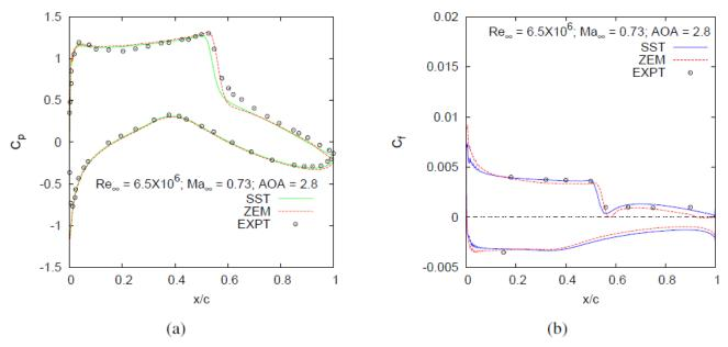
Figure 10: RAE2822 airfoil: (a) pressure coefficient profiles; (b) skin-friction profiles
