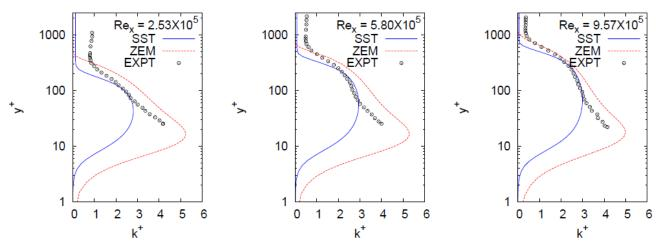
Figure 7: Kinetic energy of turbulence profiles for flat-plate at various downstream stations
