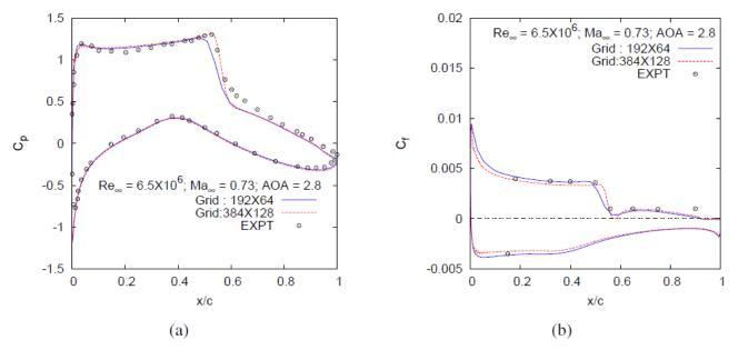
Figure 9: Effect of grid density on RAE2822 airfoil: (a) pressure coefficient profiles; (b) skin friction profiles.
