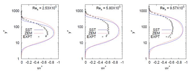
Figure 6: Reynolds shear stress profiles for flat-plate at various downstream locations
