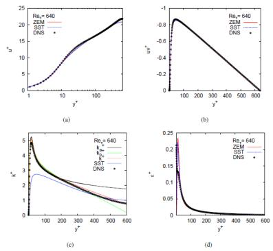
**Figure 2:** Mean profiles of turbulent channel flow  $Re_{\tau} = 640$ : (a) velocity; (b) Reynolds shear stress; (c) k; and (d)  $\mathcal{E}$
