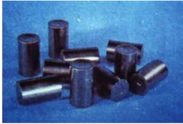
Figure 4. 10: Fuel pellets (3.5% enrichment)
