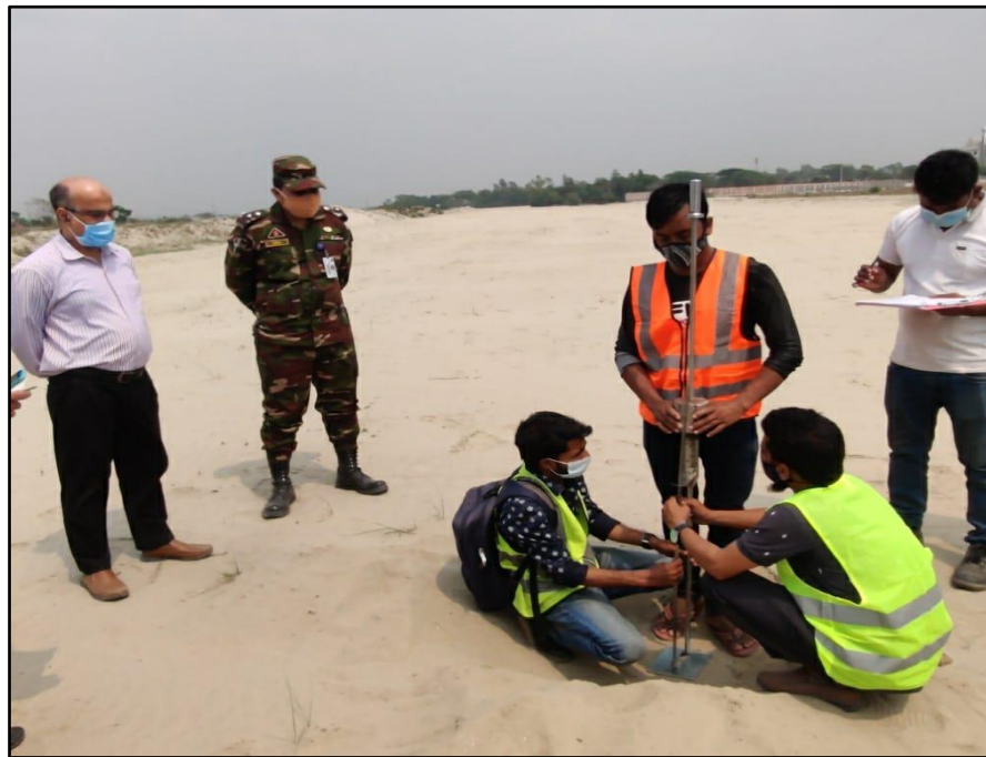
Fig. 3.5: Picture showing dynamic cone penetration test arrangements.
