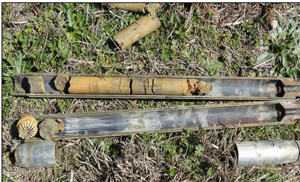
Fig 3.4: Picture of split spoon sampler with soil samples.
