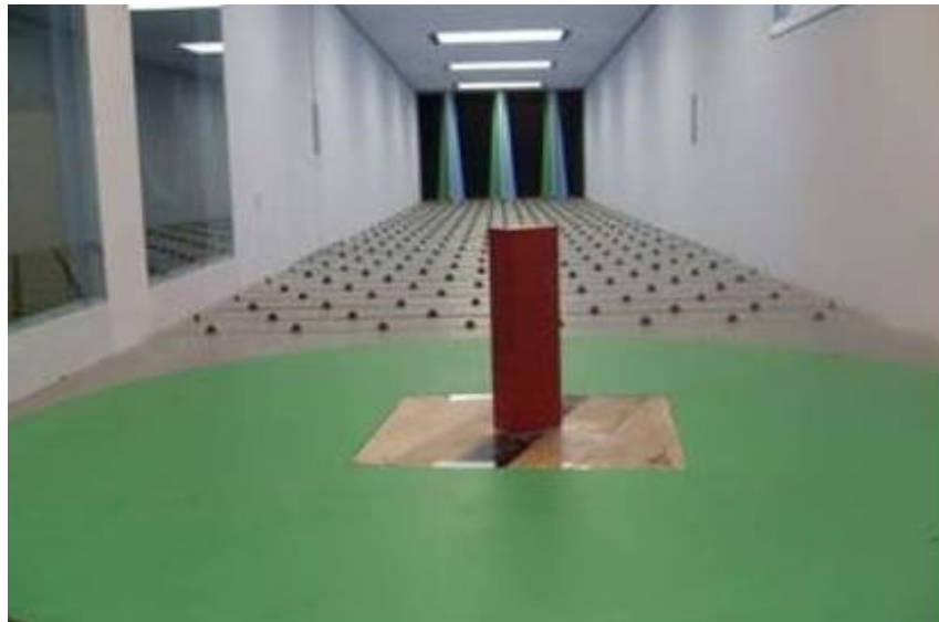
Figure 3.11: 1:400 scale model for Wind Tunnel test (Liaw, 2005)
