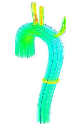
Fig. 5.33: velocity streamline.
