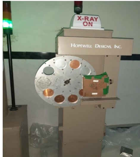
Fig. 4.1: X80-225kV X-ray Beam Irradiator
