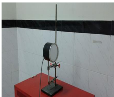
Fig. 4.2: NE2575#386 (600cc) cylindrical ionization chamber
