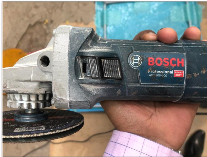
Fig: Bosch GWS 900-100 professional angle grinder with TJWELD 1.2 mm thickness cutting wheel
