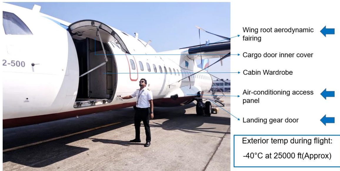
Fig. 2.9: GFRP structural components in an ATR 72-212A aircraft.
