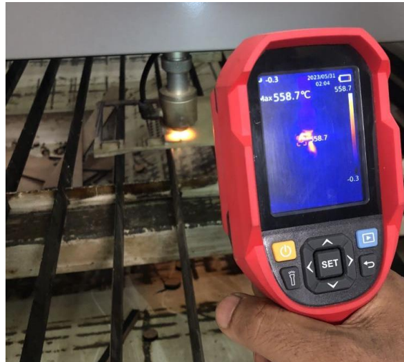
Fig. 3.5: Measurement of laser beam temperature.
