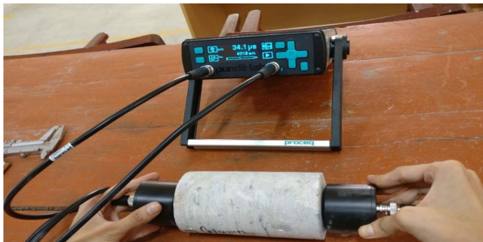
Fig 3.3: UPV data collection from the concrete core sample.
