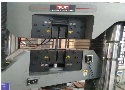
a) Rebar tensile strength test setup
