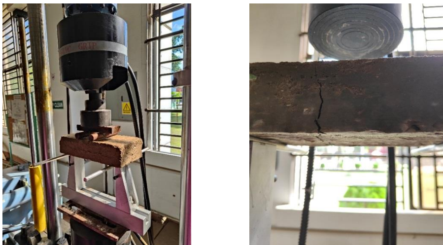
Figure 4.5: 3 rd Point Loading Flexural Strength Test
