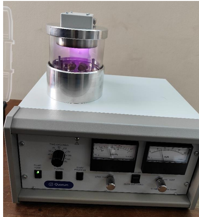
Figure 3.28: Preparation of sample for scanning electron microscopy (SEM) test
