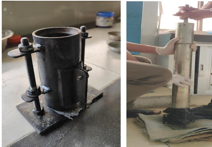
Figure 3.14: Preparation of sample for UCS test
