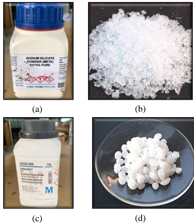
Figure 3.9: Alkali activators (a) Sodium silicates box (b) Unboxed sodium silicates (c) sodium hydroxides box and (d) Unboxed sodium hydroxides
