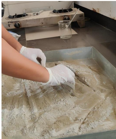
Figure 3.13: Preparation of sample for UCS test
