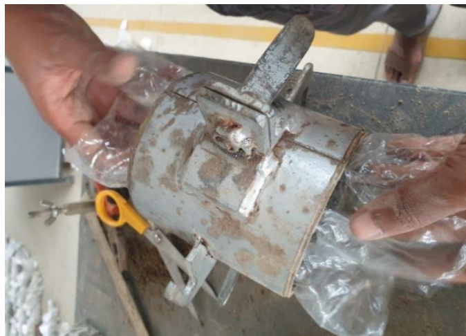
Figure 3.20: Polythene being set with the surface of the mold
