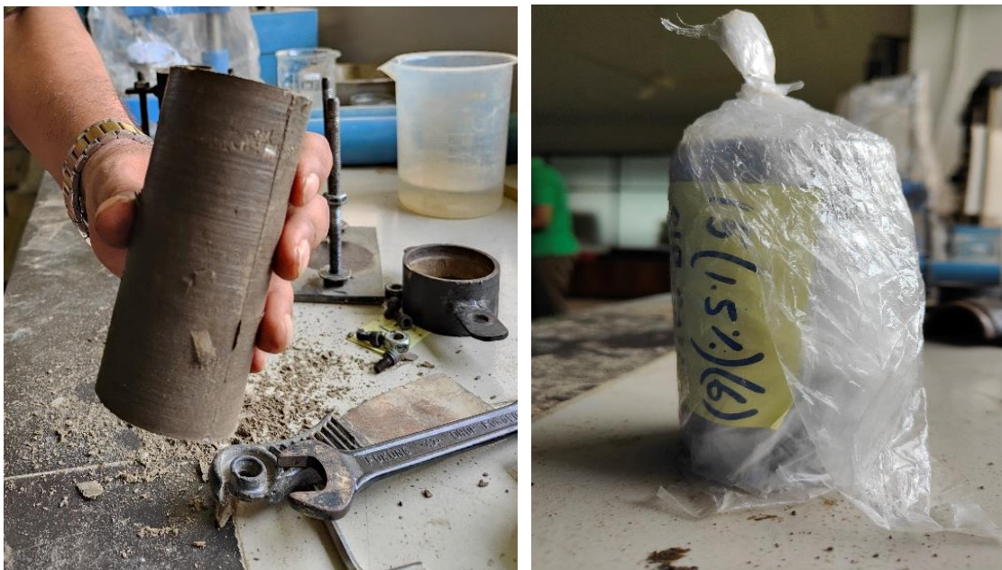
Figure 3.15: Preparation of sample for UCS test
