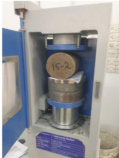
Figure 3.25: Indirect tensile strength test
