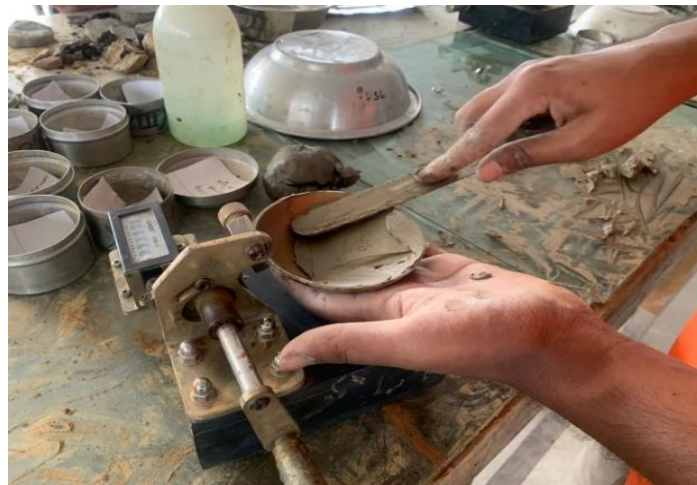
Figure 3.6: Sample preparation for Atterberg limits test
