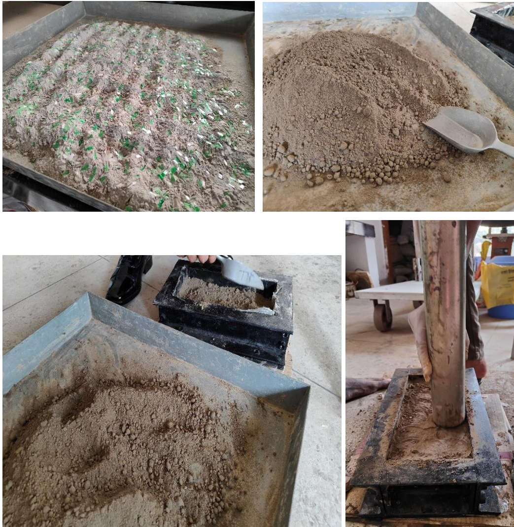
Figure 3.16: Preparation of sample for flexural strength test
