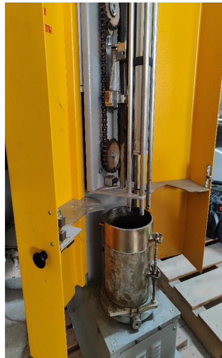
Figure 3.18: Mold preparation for CBR
