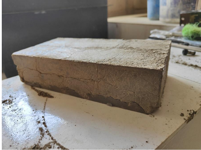
Figure 3.17: Prepared beam for flexural strength test
