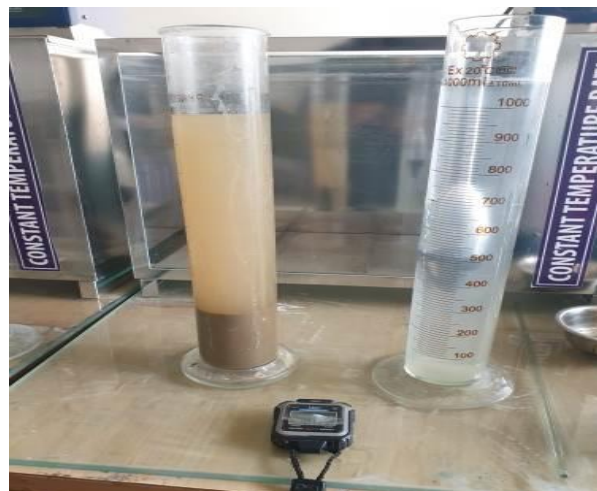
Figure 3.4: Hydrometer test of collected soil
