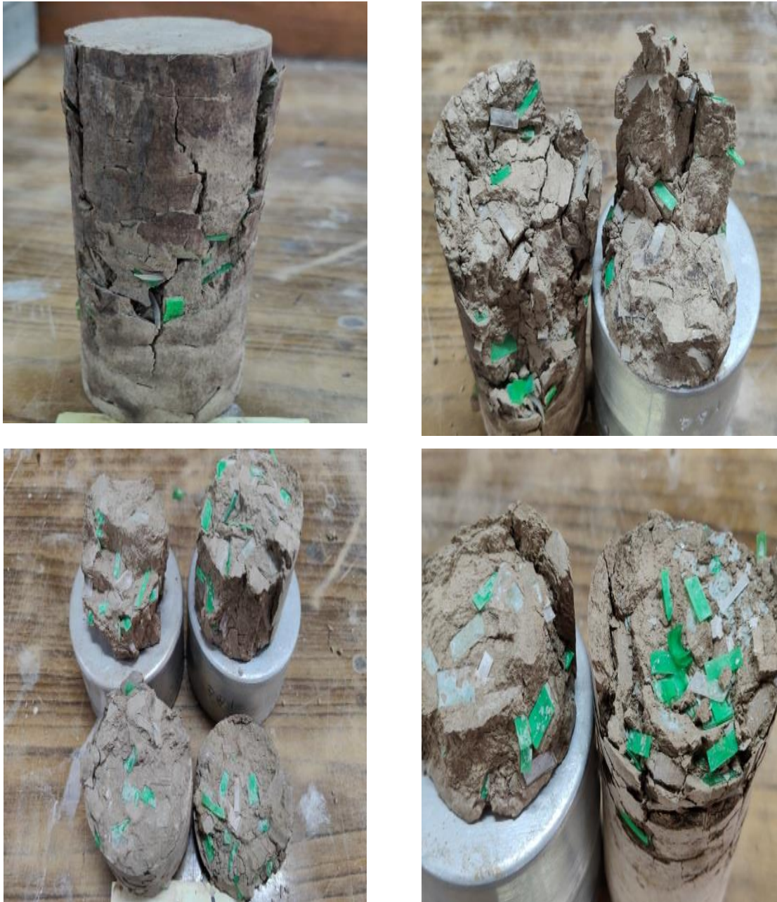
Figure 4.3: Failure planes while doing UCS test with PET strips
