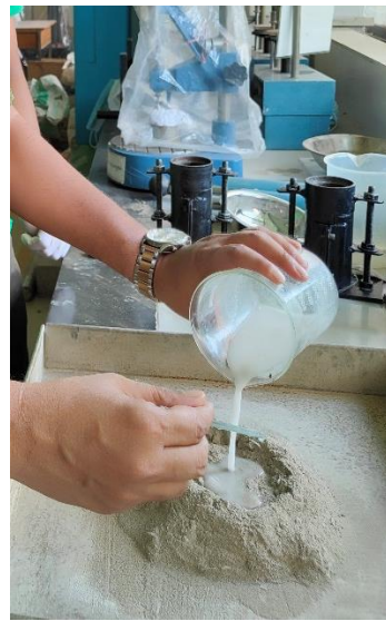
Figure 3.13: Preparation of sample for UCS test
