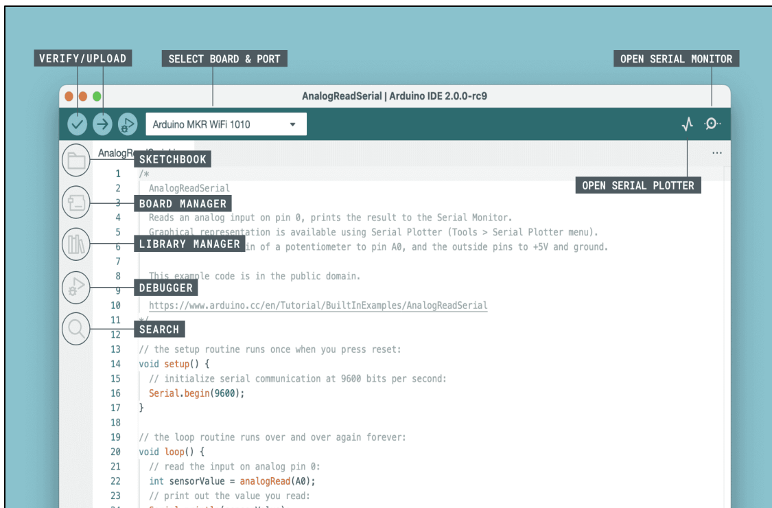
Figure 2.10: Arduino Integrated Development Environment (IDE) (Arduino, 2021)
