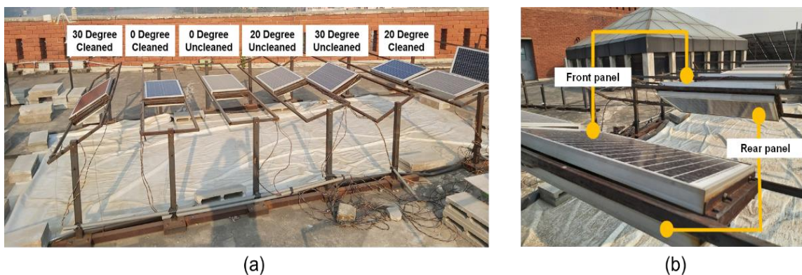
Fig. 3.10 Experimental setup of mono-facial PV panels.
