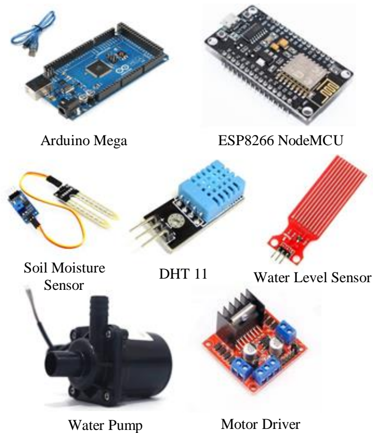
Figure 3.1: Hardware components of IoT based irrigation system
