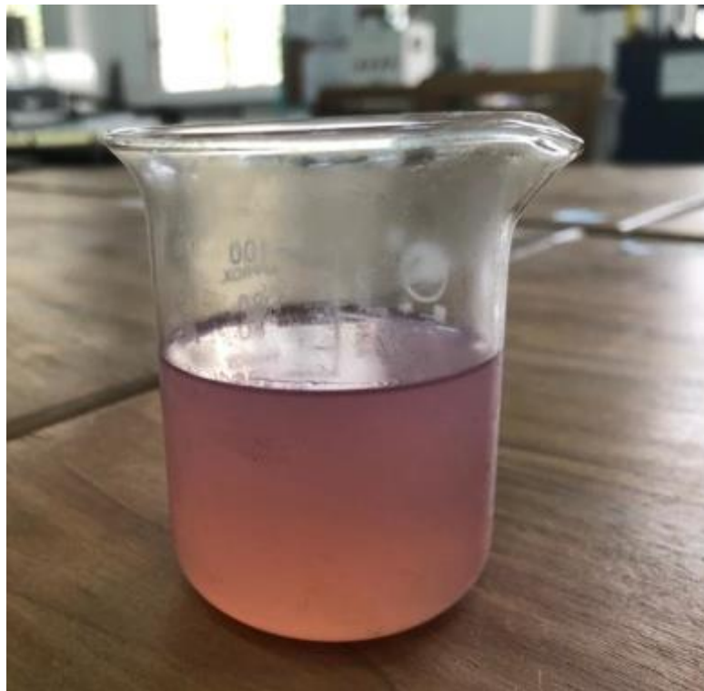
Fig 3.4: Epoxy Resin-hardener mixture
