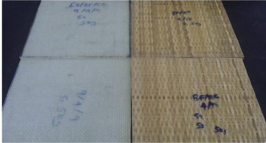
Fig 2.1: Bamboo-E glass fiber composite made by Ali et al. (2019)
