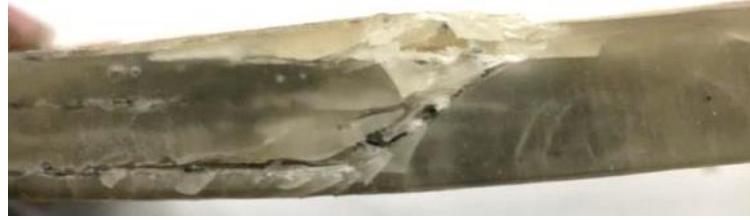
Fig 4.38: Crack Propagation of composite laminate
