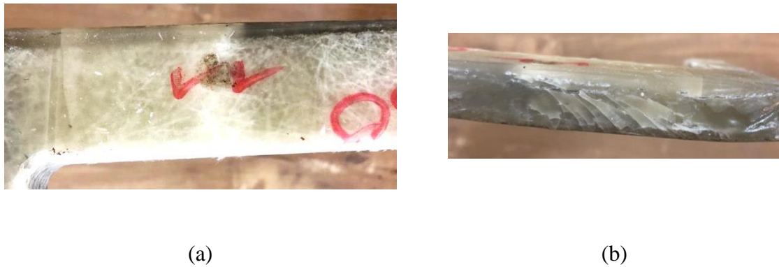
Fig 4.27: Physical condition of samples after Free fall Impact Test of (1 ply woven/ 1 ply matt) x 8 = 16 ply FG (a) Top view; (b) Side view
