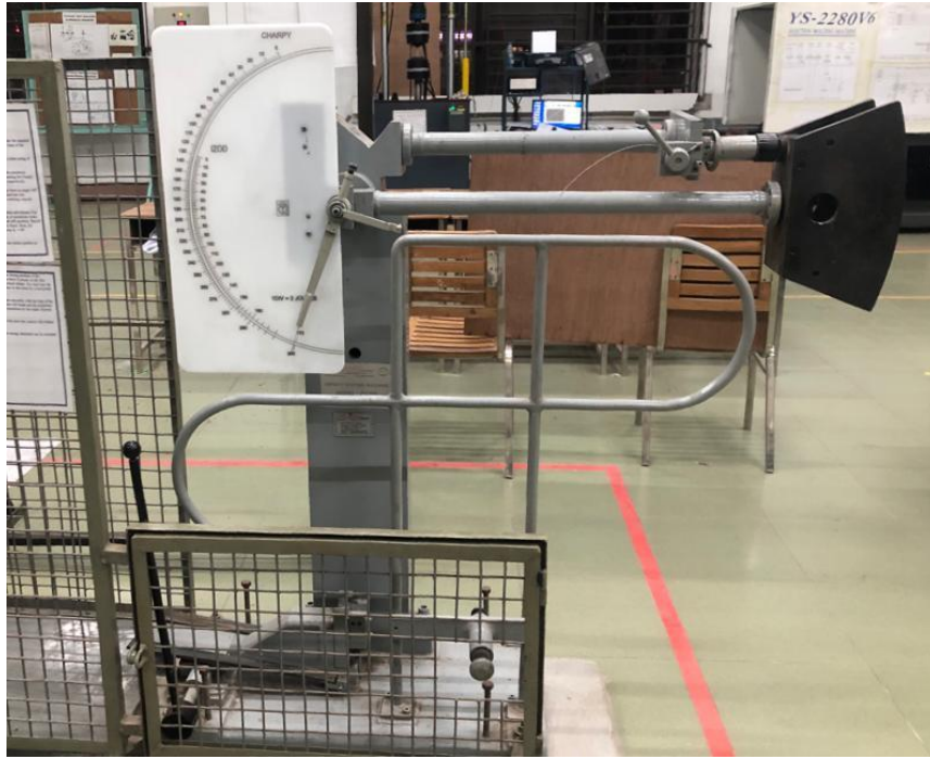
Fig 3.14: Charpy and Izod Impact Test setup
