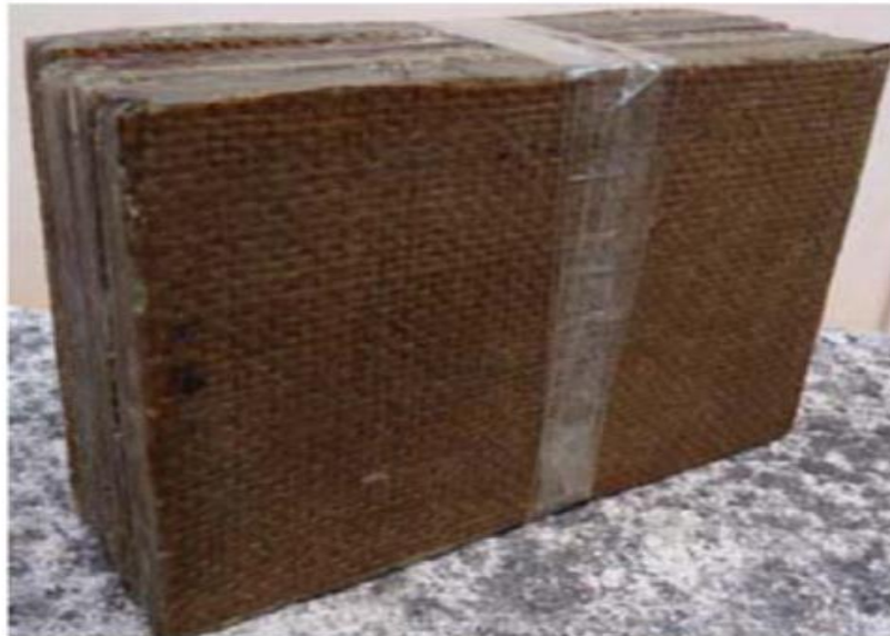
Fig 2.2: Jute/ Epoxy composite with rubber core produced by Doddamani and Kulkarni, (2012)
