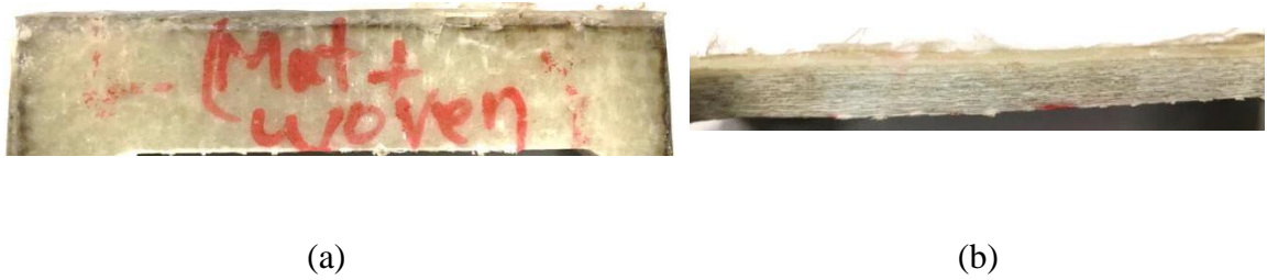
Fig 4.26: Physical condition of samples after Free fall Impact Test of (1 ply woven/ 1 ply matt) x 5 = 10 ply FG (a) Top view; (b) Side view
