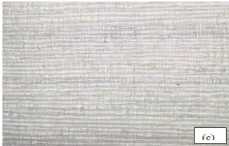
Fig 2.3: Ramie Fiber Reinforced Epoxy (RFRE) prepared by Mujiyono., Nurhadiyanto, and Mukhammad, (2017)
