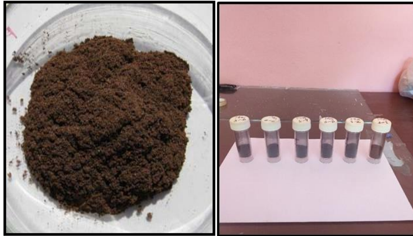
Fig. 3.3: Nano-powder of pure and Mn substituted NMCCFO.
