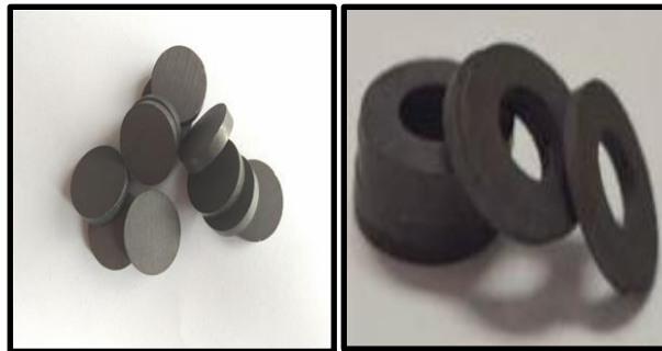
Fig. 3.4: Bulk samples of pure and Mn substituted NMCCFO.
