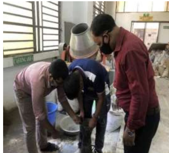
Fig 3.6 (b) Slump test
