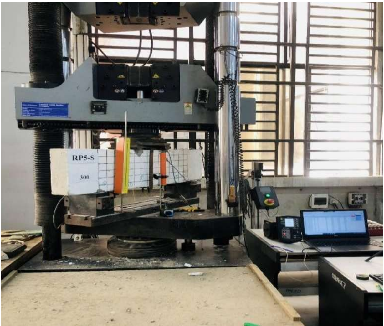
Fig 3.12: RC beam test setup and data acquisition.
