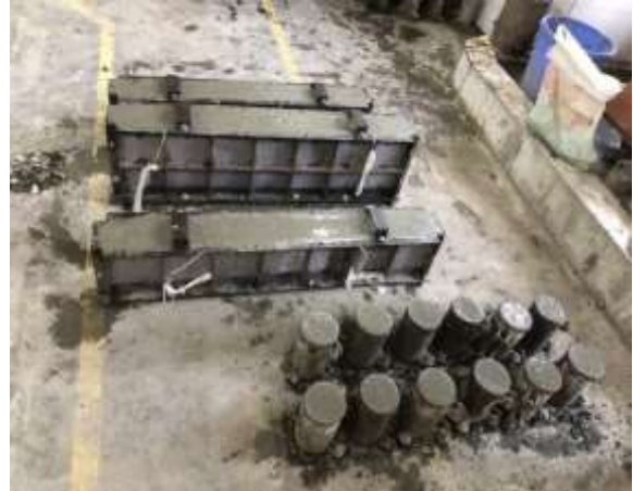
(f) Cylinder and beam casting
