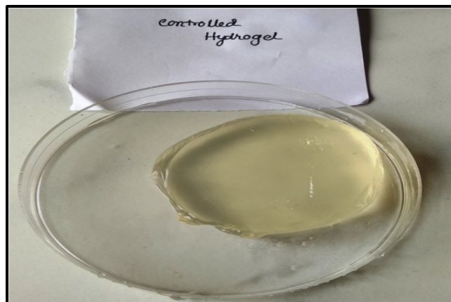
Fig. 3.4: NH Dressing Material (contain only PVA & Gelatin)
