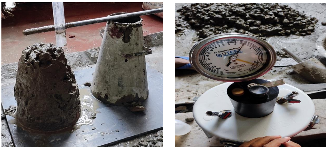
Fig.3.3 (a) Slump test of Concrete mix (b) Air Content test of Concrete mix
