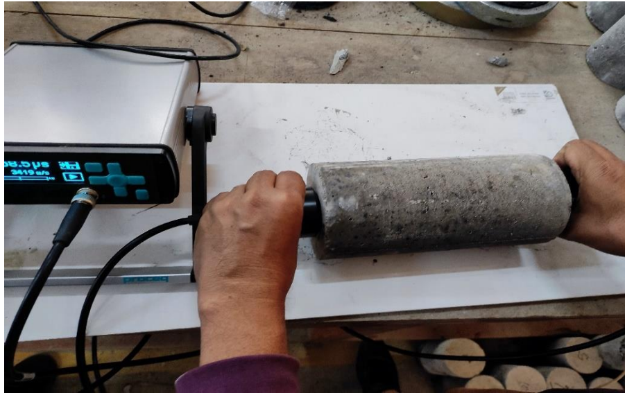
Fig 3.9: UPV test of cylindrical specimen
