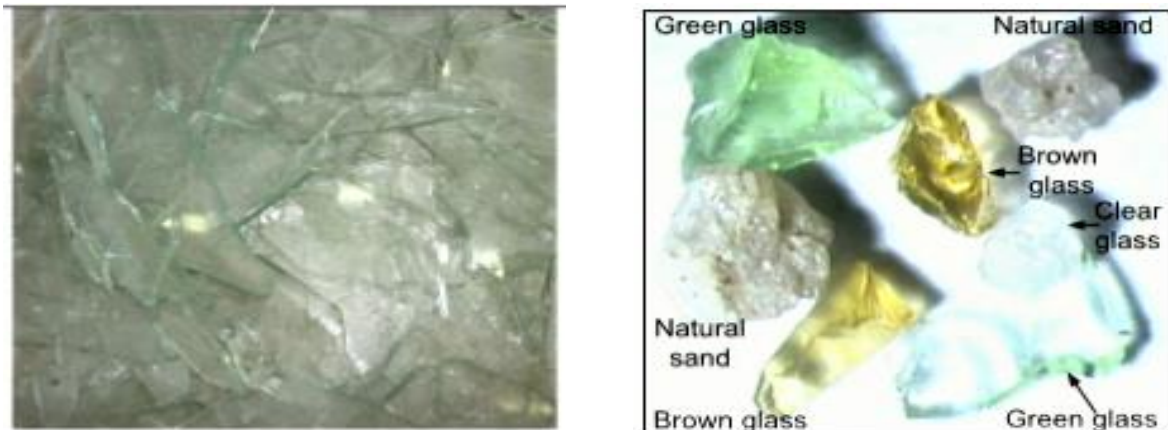
Fig. 2.2 Crumb Glass (a) appearance of natural and glass sand (b) flat glass
