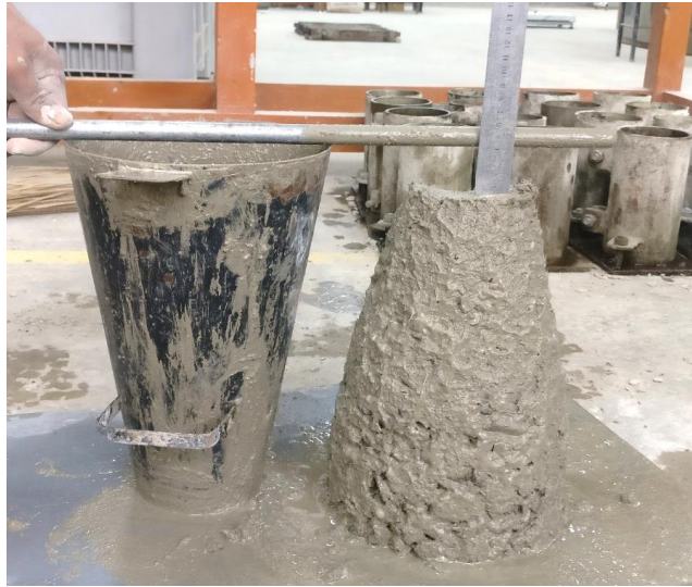
Fig. 2.5 Typical slump test of concrete (Jia et al., 2015)
