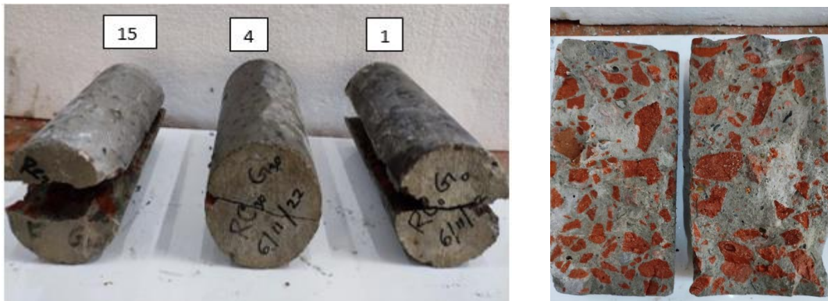
Fig. 4.18. (a) Failure pattern of RCG concrete cylinder in tension (b) cross section after failure
