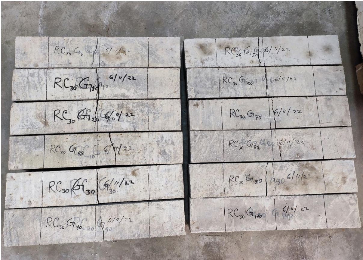
Fig. 4.20. Flexural failure pattern of RCG concrete
