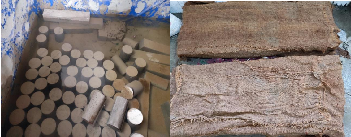
Fig.3.7 Curing process of cylindrical, prism beam and reinforced beam specimen
