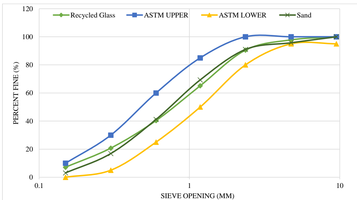
Fig 3.2: Particle Size Distribution Curve of WG and Natural Sand
