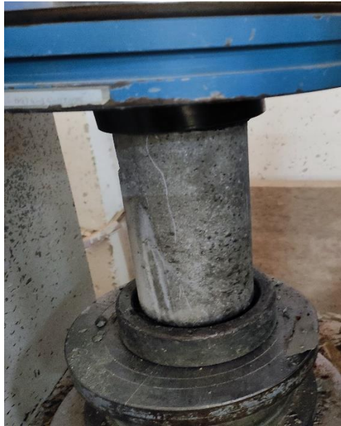
Fig. 3.8: Compression test setup of Cylindrical specimen
