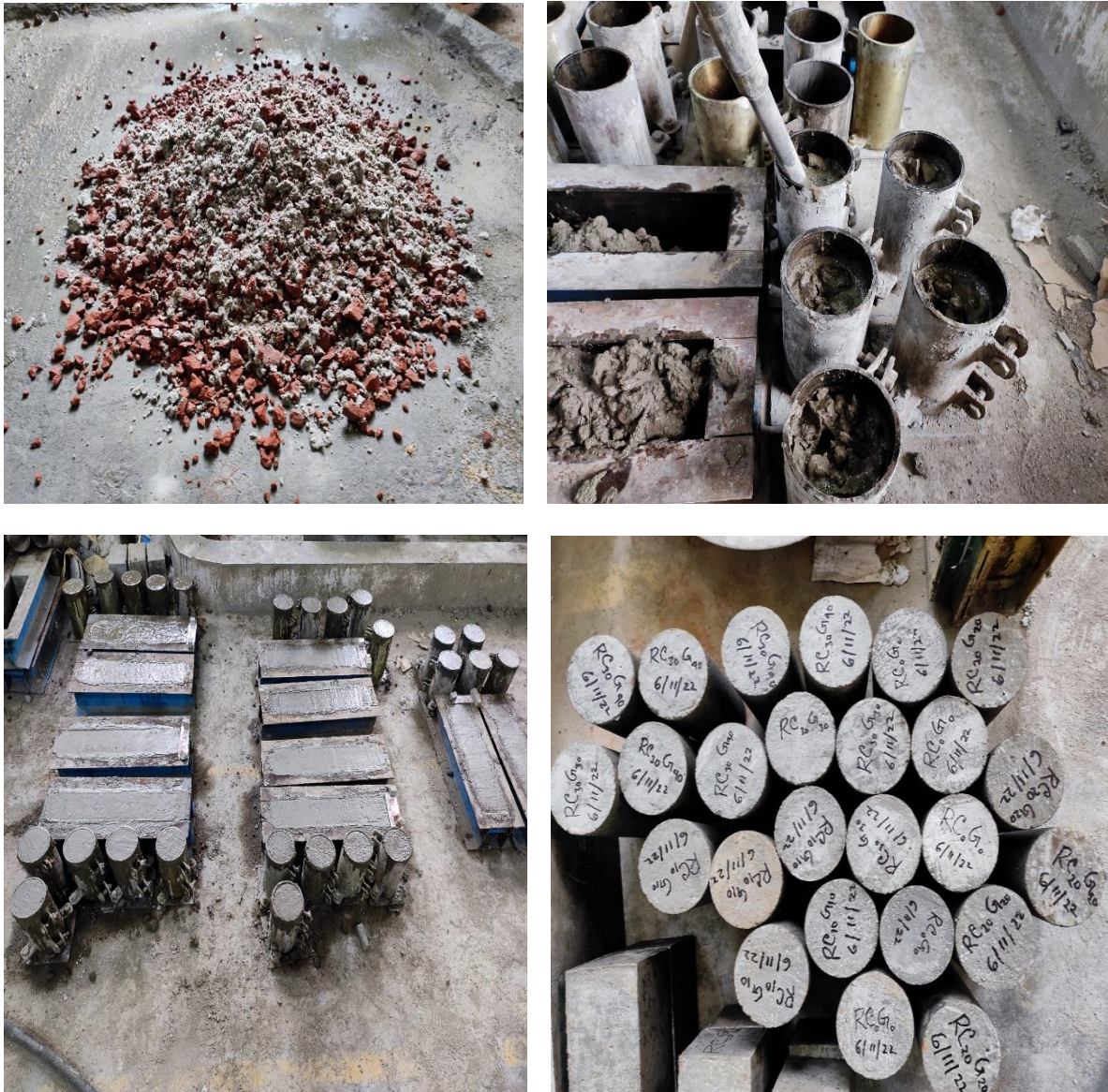
Fig.3.4 (a-d) Mixing, Hammering, Casting and Notation
