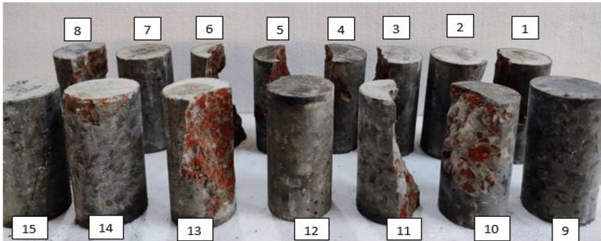
Fig. 4.17. Failure pattern of RCG concrete cylinder in compression
