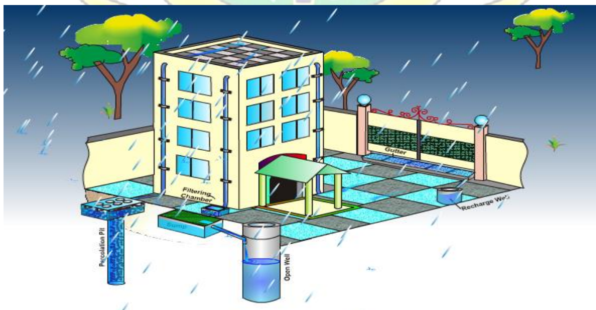
Rainwater Collection in Multistoried Roofs
