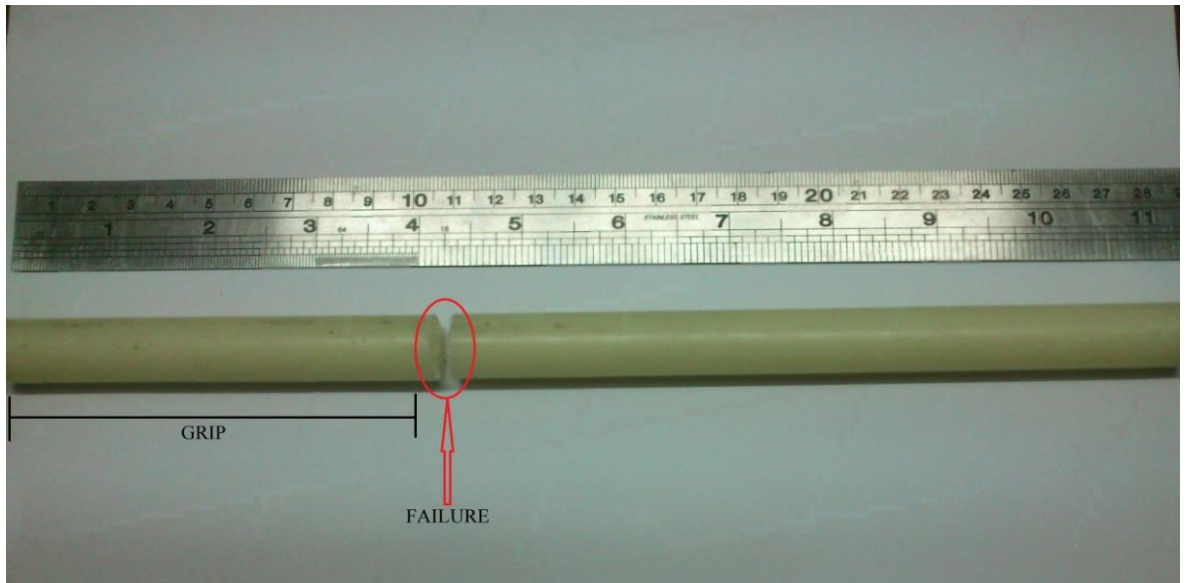
Fig: 2.1.3 Initial failure in the circular rod specimen
