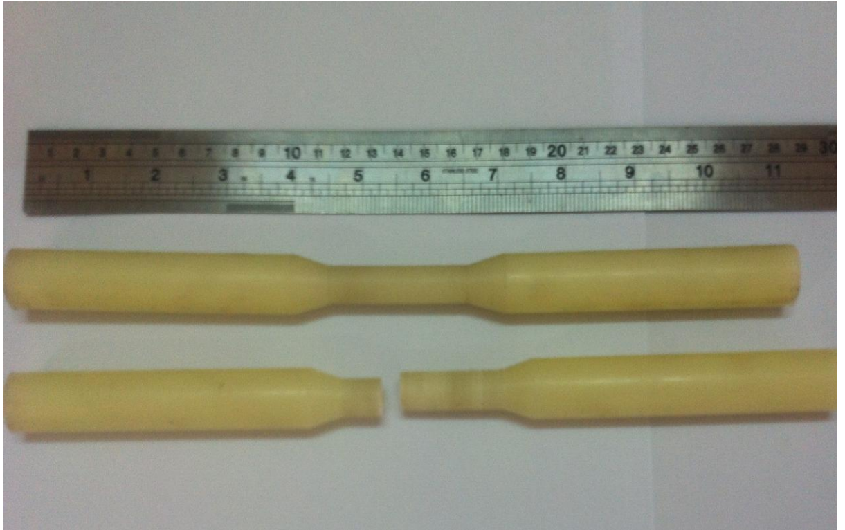
Fig: 2.1.7 Modified machined specimen with failure part
